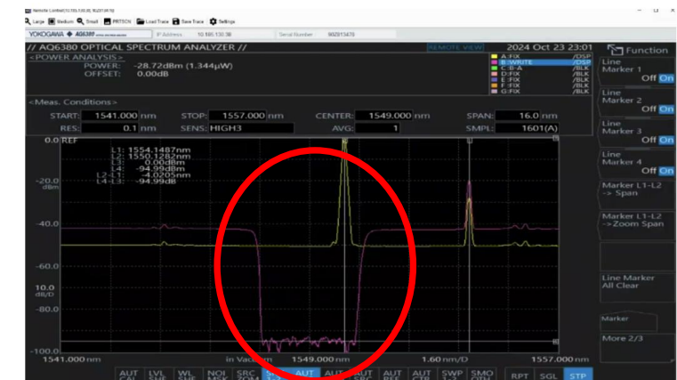
(b) Probe signals measured at the output of the 5-filters cascade.
